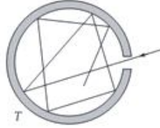
(Figure 2.1: Model of the blackbody)
