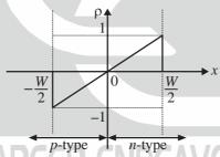
The figure that best depicts the variation of the electric field E with x is (W denotes the width of the depletion layer, and electric field is zero outside the depletion layer).
